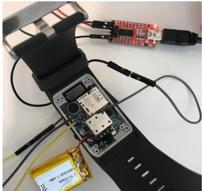
*Figure 2. Assessing debug interfaces on the Tinitell.*
